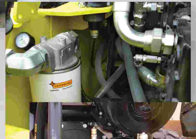
Location of hydraulic filters, hydraulic pumps with pressure inlets, more accessibility and easier.
