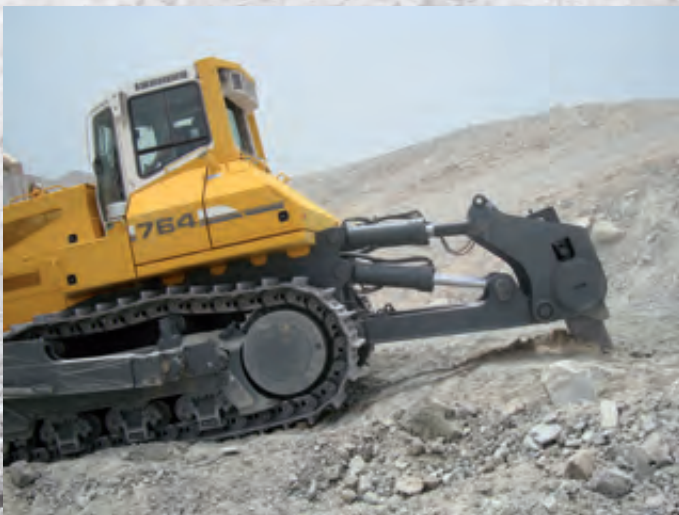
Best all round vision as a result of integrated ROPS/FOPS protection
