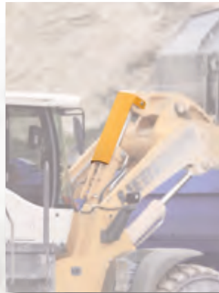
Piston rod protection for tilt cylinder optional
