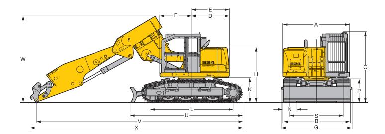
with Boom 3.03 m,  $2 \times 45^{\circ}$  Rotator and Stick 3.20 m
