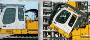
Demolition cab, 30° tiltable for an excellent view of the working area and fatigue-free working (optional)
