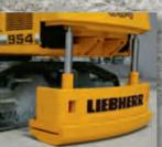
Counterweight can be hydraulically lowered for lowering the weight during transport
