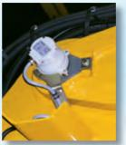
One of three LDC sensors on the attachment for permanent monitoring of the equipment position
