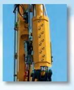
Piston rod protection for tilting cylinder prevents damage to the cylinder
