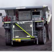
The T 264 features high-powered, frictionless dynamic braking. The AC drive system delivers up to 3,300 kW (4,425 HP) of electric dynamic braking, reducing engine loading and fuel consumption.
