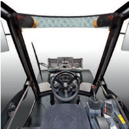
Optimum front and rear view due to monoboom and compact rear end
