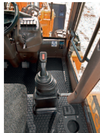
Easy handling; nearly all operating functions are integrated in one joystick
