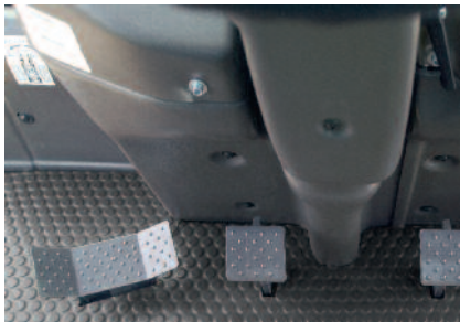
Left foot operated swing pedal avoids tiredness
