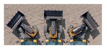
The slender monoboom increases the working area between the wheels by 32%
