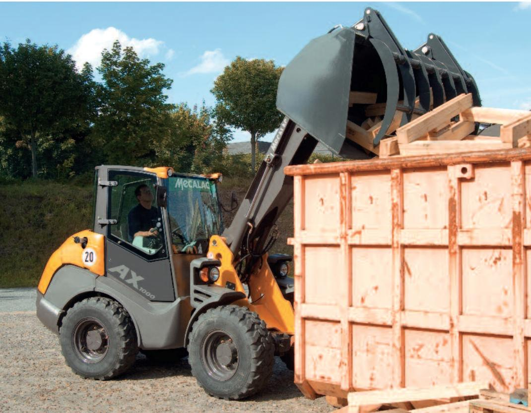
**Due to the monoboam,** the Mecalac AX features high breakout forces. Its Z-kinematics allow for perfect parallel guidance of attachments. This results in a high degree of safety, in particular when loading pallets. Fast tipping cycles and an excellent view on the attachments make daily work even more efficient.
