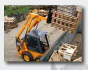
**COMPACT** Iow-profile design and minimal width of 48.4 inches makes working in small spaces easy. Low overhead height of 70.3 inches with standard tires allows entrance into low-clearance buildings.
