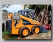
STURDY A Level II-certified **ROPS/FOPS** structure provides protection, yet allows an unobstructed view to the attachment and surrounding work areas.
