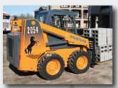
MOVE MORE A with an operating capacity of 1,750 lbs. (with optional counterweight) for exceptional lifting and loading capabilities.
