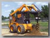
STURDY ▲ Level II-certified ROPS/FOPS structure provides protection, yet allows an unobstructed view to the attachment and surrounding work areas.
