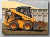
are made possible with the optional hydraulic MultiTach™ attachment system allows the operator to change attachments without leaving the seat.
