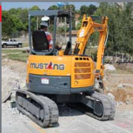
**TRUE ZERO-TAIL-SWING** ▲ Innovative design ensures that the upper structure never overhangs the tracks. Cast side protectors guard and prevent damage to the machine.
