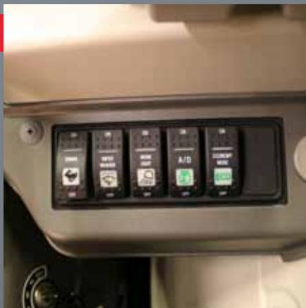
**ECO MODE** ▲ Activated by the flip of a switch, ECO mode reduces engine speed by 10% without sacrificing power, saving fuel when full speed is not necessary.
