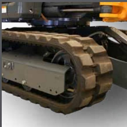
**STABLE TRACKS** ▲ Wider track gauge and offset track drive system increase stability without adding to the overall machine width.
