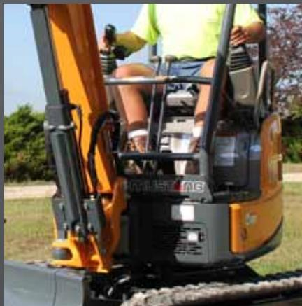
**EXTRA PROTECTION ▲** Bucket, dipper and boom cylinders are protected by plate spring cylinder guards, while the upper structure lower frame corners are reinforced by high-strength steel covers.
