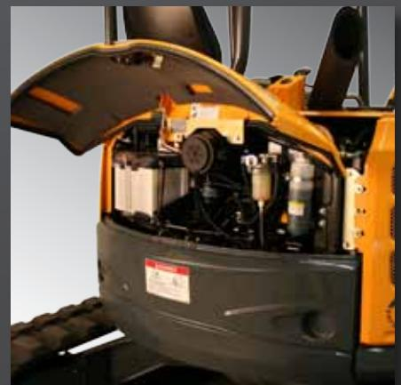
**EASY SERVICE ACCESS** ▲ Large, rear hood opens easily to expose the battery, engine oil, air filter and cooling system.
