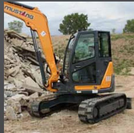
**ZERO-TAIL-SWING** ▲ Zero-tail-swing design allows the superstructure to rotate entirely within the tracks without overhang, allowing operation close to walls and other obstacles.
