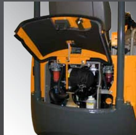
**SERVICEABILITY ▲** Removable side panels, a large rear door and access panel under the operator seat provide the access needed for hassle-free serviceability and daily maintenance checks.
