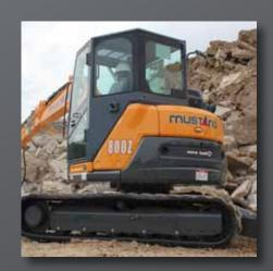
AUTO DECELERATION A This function improves fuel economy and lowers noise and emissions levels by reducing engine speed to idle after four seconds without hydraulic movement.
