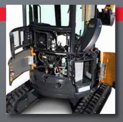
Two large rear doors, a swing-open side access panel, and removable covers beneath the operator's seat provide ample service access.
