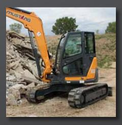
**ZERO-TAIL-SWING** A Zero-tail-swing design allows the superstructure to rotate entirely within the tracks without overhang, allowing operation close to walls and other obstacles.
