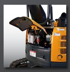
**EASY SERVICE ACCESS** Large, rear hood opens easily to expose the battery, engine oil, air filter and cooling system. Right-hand side cover easily removes for access to the radiator.
