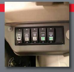
**ECO MODE** A Activated by the flip of a switch, ECO mode reduces engine speed by 10% without sacrificing power, saving fuel when full speed is not necessary.
