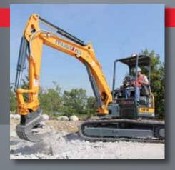
HYDRAULIC FLOW ▲ Four hydraulic pumps provide the ample flow required for smooth operation, even while using the boom and arm simultaneously.
