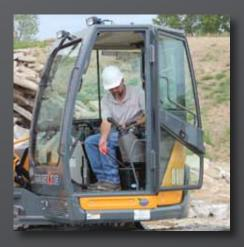
OVERSIZED CAB Large cab provides a spacious, ergonomic operating environment. The cab is mounted on five silicon oil-filled iso-mounts, which reduce cab noise and vibration to the operator.
