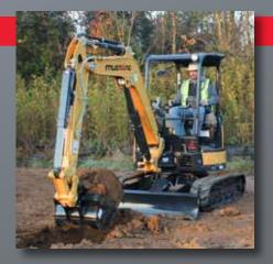
POWERFUL ▲ Yanmar Tier IV emissions certified 24.4 hp (18.2 kW) diesel engine provides 20% less fuel consumption and an electronic throttle for precise control.
