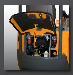
**SERVICEABILITY** A Removable side panels, a large rear door and access panel under the operator seat provide the access needed for hassle-free serviceability and daily maintenance checks.
