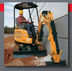
**ZERO-TAIL-SWING** A True zero-tail-swing design, paired with cast side protectors, offers protection when working near a variety of structures and obstacles.
