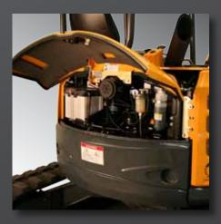
**EASY SERVICE ACCESS A** Large, rear hood opens easily to expose the battery, engine oil, air filter and cooling system.
