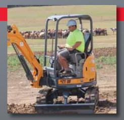
TRUE ZERO-TAIL-SWING A Innovative design ensures that the upper structure never overhangs the tracks. Cast side protectors guard and prevent damage to the machine.
