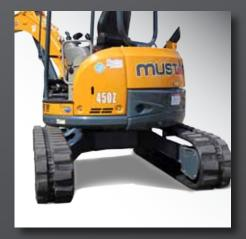
**EXTRA STABILITY** Wider track gauge and offset track drive system enhances machine stability without adding to overall width.
