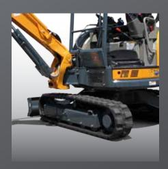
EXTRA STABILITY A Wide track gauge and offset track drive system enhance machine stability without adding to overall machine width. Angled crawler frame reduces soil buildup.
