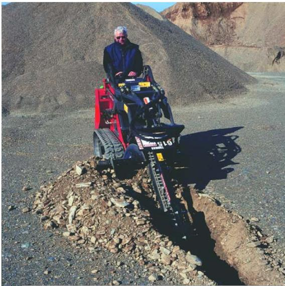
When high speed travel is not required and you are operating attachments that require high hydraulic such as snow blowers and trenchers, flow and power can be switched to the auxiliary hydraulic circuit.
