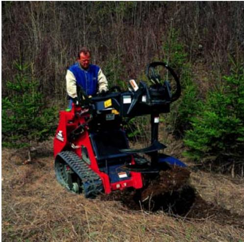
For the protection of rotating motor powered attachments such as sweepers, tillers, power box rakes or snow blowers there is a second circuit equipped with built in motor spool. The motor spool protects the attachments motor from pressure surges and spikes caused when hydraulic flow is reversed or shut off. When operating a sweeper for example the motor spool will allow the brush to free spool when hydraulic flow is shut off.
