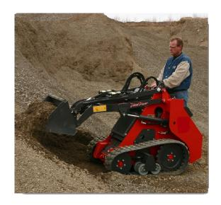
Unlike most of its competitors the 45DTN is not just a simple lift and carry machine. This loader gives you true digging and excavating performance.
