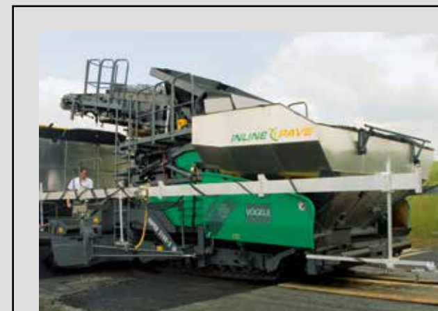
7 Using the lifting gear, two workshop staff members raise the InLine Pave transfer module onto the SUPER 2100-2 IP, positioning it in place and securing it. Then they fit the muffler end pipe.
