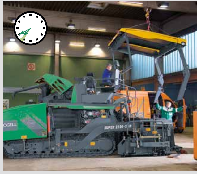
2 Conversion begins with removal of the paver's hardtop and the muffler end pipe.
