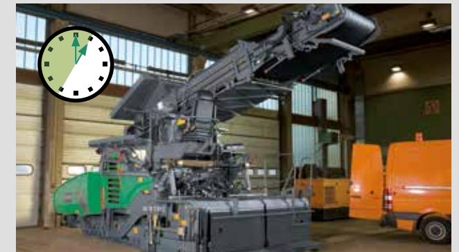
8 Finally, hydraulics and electrics are connected. A test run should be performed, checking all components for proper functions and making final adjustments.
