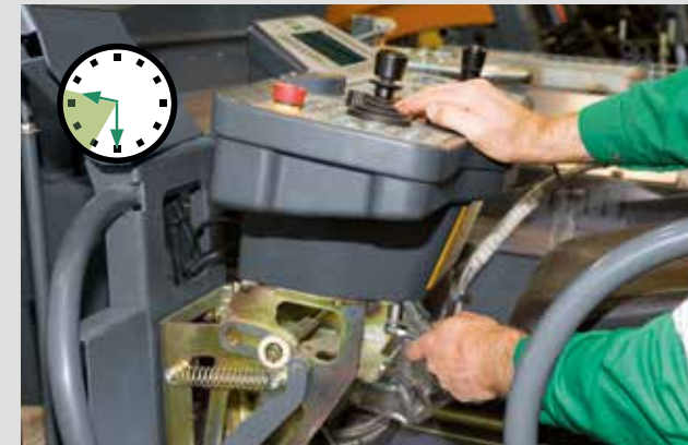
5 The ErgoPlus operating console is fitted on the operator station of the InLine Pave transfer module. Electrical cables are connected.
