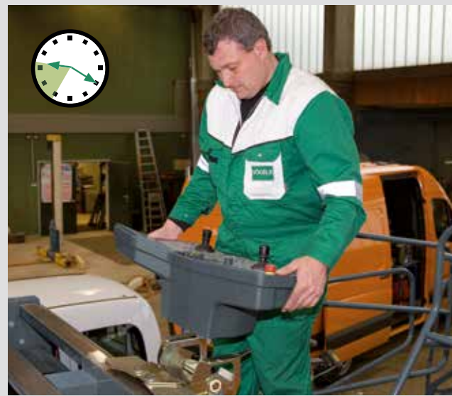
4 Then the ErgoPlus operating console is taken off, including slide rail.
