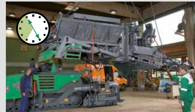
7 Using the lifting gear, two workshop staff members raise the InLine Pave transfer module onto the SUPER 2100-2 IP, positioning it in place and securing it. Then they fit the muffler end pipe.
