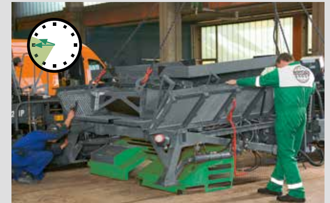
6 Before lifting the transfer module onto the paver, the engine hood has to be attached.
