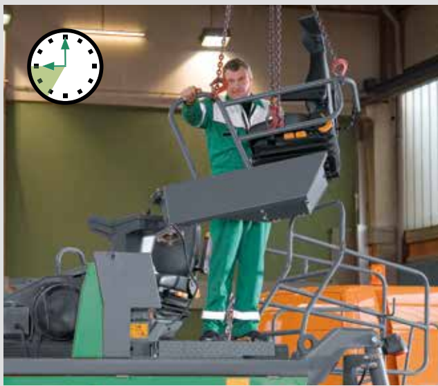
3 Next is removal of the engine hood, the driver's seats and the guard rails.
