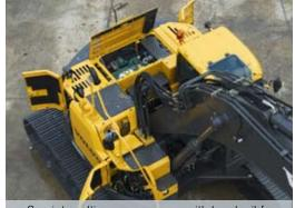
• 3-point, multi-purpose access with hand rail for ease and safety.
