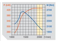
Ideal characteristic curve: the engine output remains constant even at extreme engine lugging
