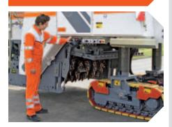
The scraper blade can be swung open hydraulically for cutting tool replacement
