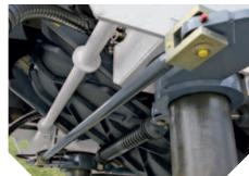
Working independently of the level selected, the parallel sliding block guide ensures precise steering
