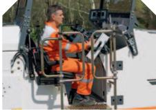
Both control panels can be moved out over the edge of the machine
