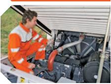
Ample space for maintenance provided by the wide-open engine cowling
