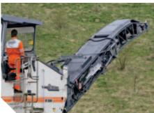
The discharge conveyor can be raised hydraulically
