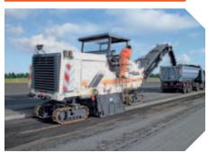
▲ The W 2000 large milling machine efficiently removes complete road pavements ...
