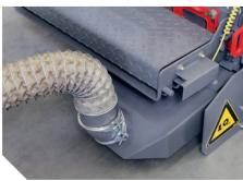
A separate suction port has been provided at the rear of the machine
