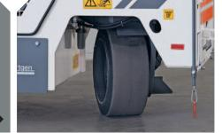
Large locking angles of the front wheel permit small milling radii
